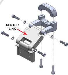
5 - The center-link may be removed if an overall shorter mount length is needed, depending on your rear view miror and desired position for the RD. With multiple adjustments available, you should be able to postion your RD right where you want it. If you are unable to achieve this, be sure to contact us at 1-707-664-8234
